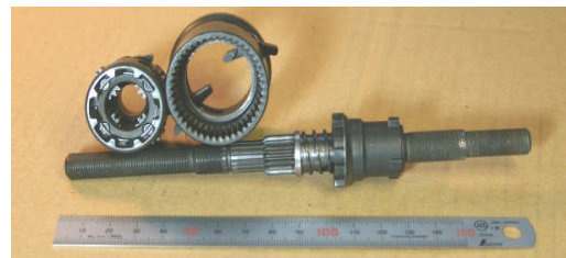
(b) Main parts for planetary gear drive ( m0.8, z_s=15, z_p=14, z_r=45 )
